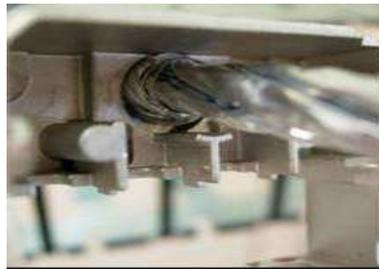
Release the cable clamp when it is pressing both jacket and braid
