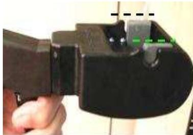
Make sure the Tool Adapter for AMP CO is fully inserted into the Pistol Grip Tool, as shown
