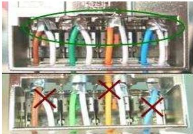
Carefully check from the back the correct position of the wires over the SEC IDC blocks (re-arrange the wires if necessary) and the correct position of each pair's foil: wrapped around the wires and as close as possible to the IDC block
