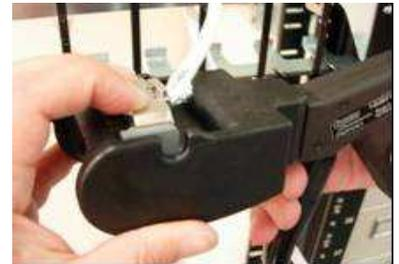
Insert up to the limit the rear housing group into the Pistol Grip Tool and terminate the wires with the Tool
